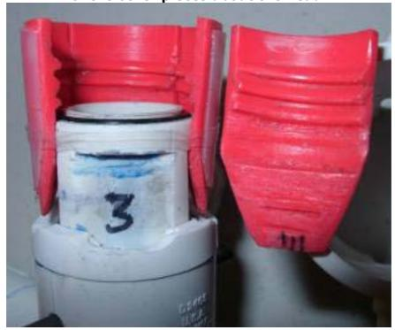
The four red collet pieces were originally a <u>Tornado Tube</u>®—my Dremel tool brought about the transformation. With the trigger ring in place, the force of the pressurized bottle cannot pull the collet pieces out of the head unit, due to mutually opposing ledges between the "bare" head and collet pieces.
