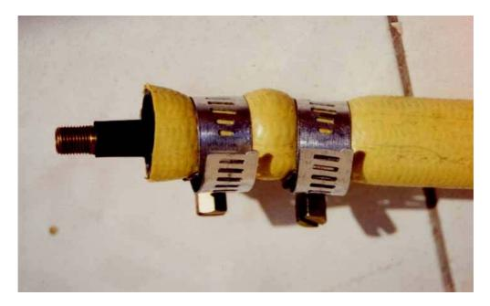
This is the garden hose with the two clamps holding the tubeless tire valve in place.
